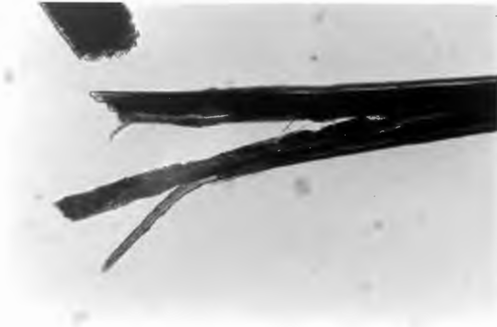
Figure 4.8. Whole mount of fibre from sample no. 1, showing the split end at the tip. Magnification 120x.
