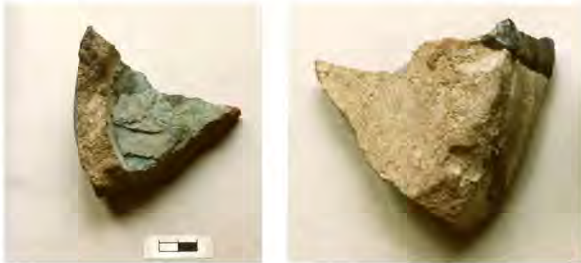
Figure 10.14. Top and underside of sagger containing laminated substance (? malformed frit). The underside shows splash-mark of glass. The scale bar is 2 cm. Petrie Museum, UC 36858. Photograph by courtesy of the Petrie Museum, University College London.
