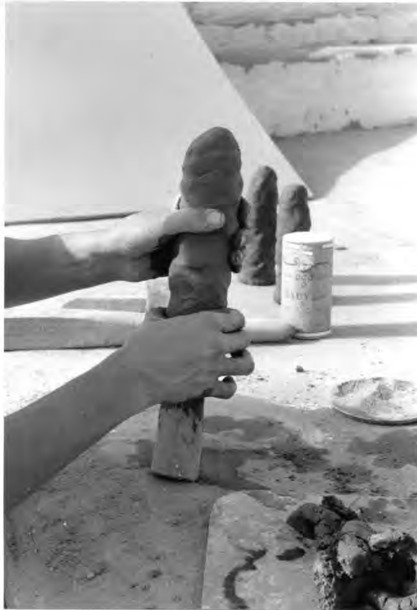
Figure 11.5. Pressing clay around a patrix whilst it is rotated.
