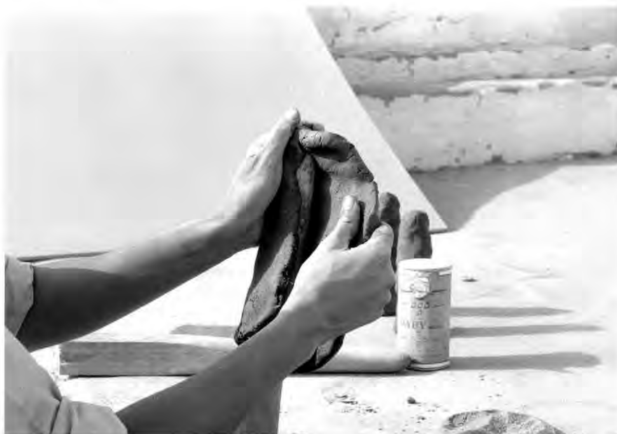
Figure 11.4. Wrapping clay around a patrix .
