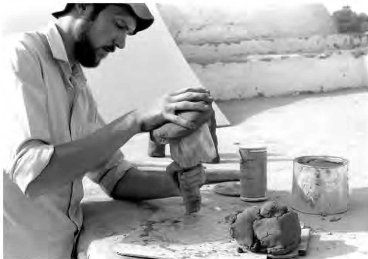
Figure 11.6. Putting clay on to a hemispherical patris .
