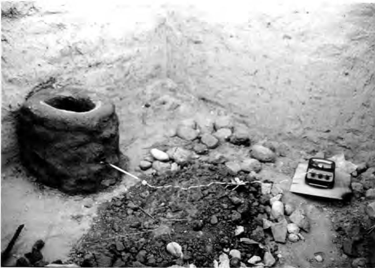
Figure 12.7. Replica oven with thermocouple in position.
