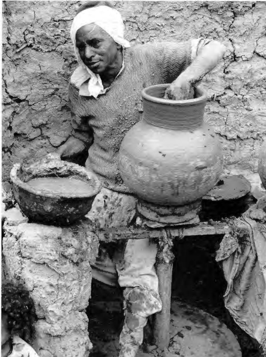
Figure 9.11. Drawing up the rim into a flaring neck by revolving the wheel sufficiently to use centrifugal force.
