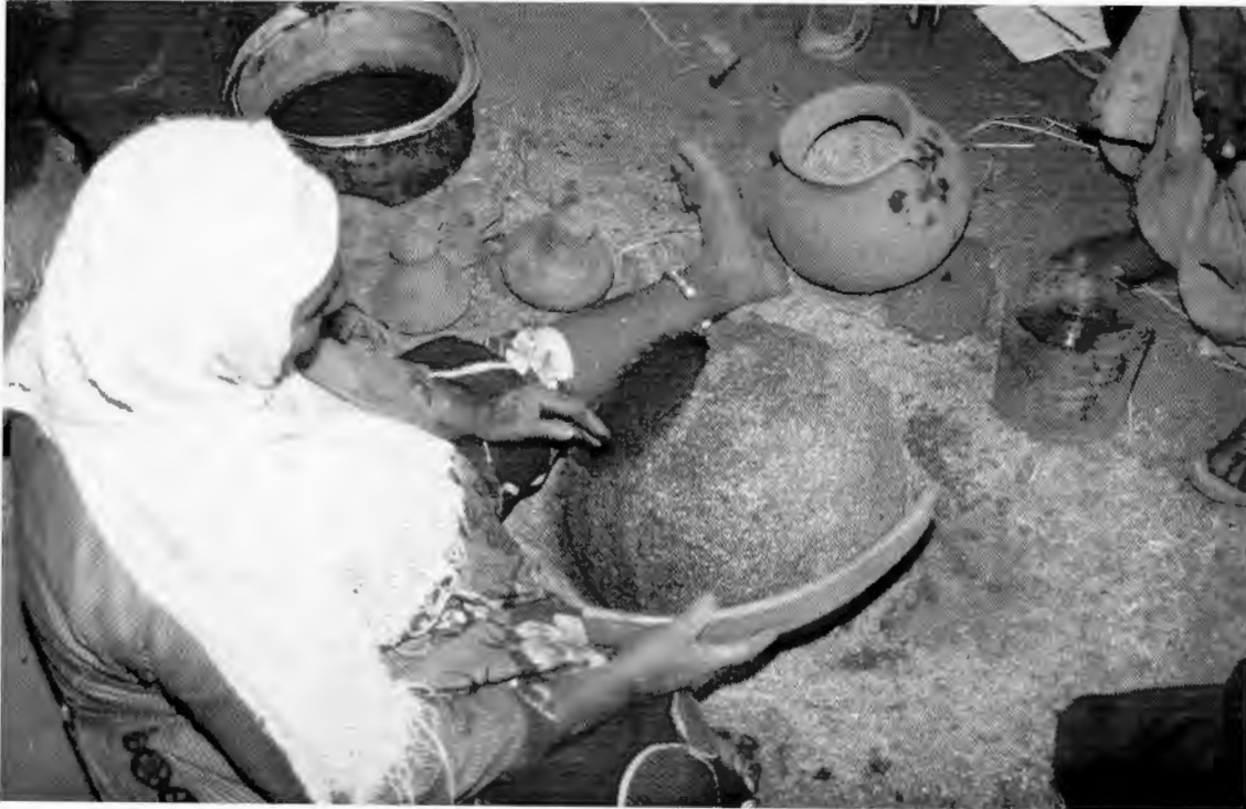
Figure 9.6. The “pie-crust” rim is checked and repaired to strengthen the vessel during the thinning with the paddle.
