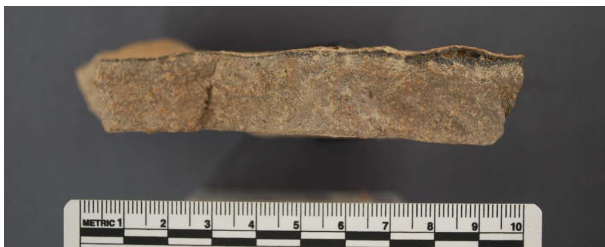
Figure 2: Cylindrical vessel base 40348 showing the vitrification layer below the parting layer. Photo: A. Hodgkinson.
